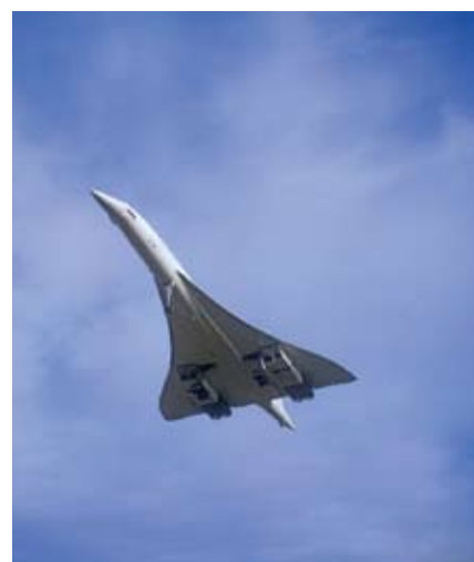
Figure 7.18 When Concorde flew at over twice the speed of sound, it got so hot that it increased its 61.6 m length by about 30 cm.
