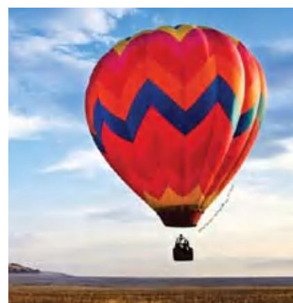
Figure 6.47 The buoyant force from the air keeps the hot balloon in the air.
