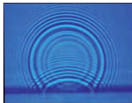
Figure 8.32 Ripples in a ripple tank reflect off a straight barrier
