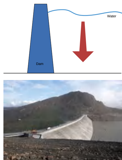
Figure 6.27 Dams have to be thicker at the bottom in order to withstand the greater pressure.
